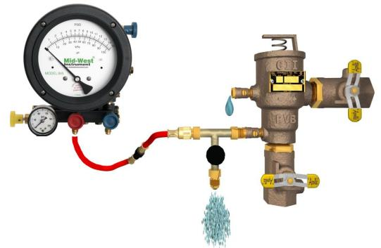
The 830-0001 has a soft seated needle valve, a quick coupler for connection to a  $\frac{1}{4}$ " flare fitting at the test cock and a flare connection for connection of the test kit hose to the assembly.
